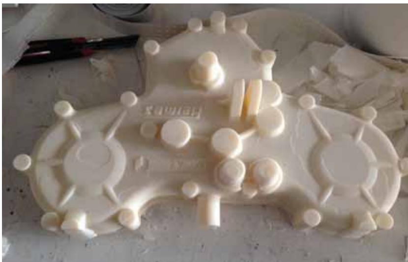
Model vytiskný metodou FDM fused deposition modeling.
