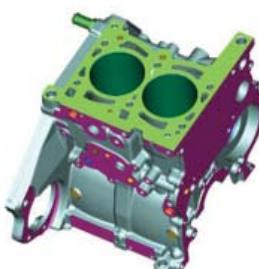
Obr. 3 Blok motora TwinAir z liatiny [3]
