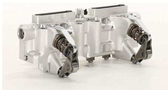
Obr. 16 MultiAir modul motora TwinAir [14]
