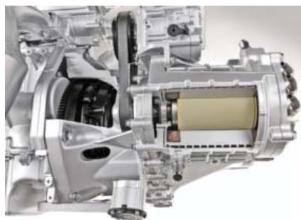
Obr. 11 Rez prevodovkou HDDCT s elektromotorm [8]
